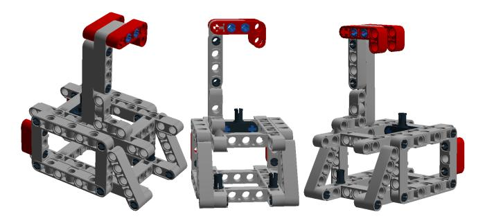
There are 3 pods. Each pod weighs 50 grams. One pod contains an additional weight of about 69 grams representing the hockey bag. The weight is made of a non-ferromagnetic metal material, copper. It is made from 3 plumbing sleeves of 19mm in diameter (¾" coupling). The sleeves are flattened with a hammer and held with tape.
