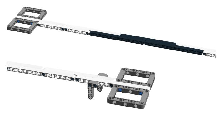
The rail is made of 24 15-hole beams and frames at the ends. The frames at the ends are firmly attached (screwed) to a wooden support. The other end is placed on a support made of LEGO bricks.
